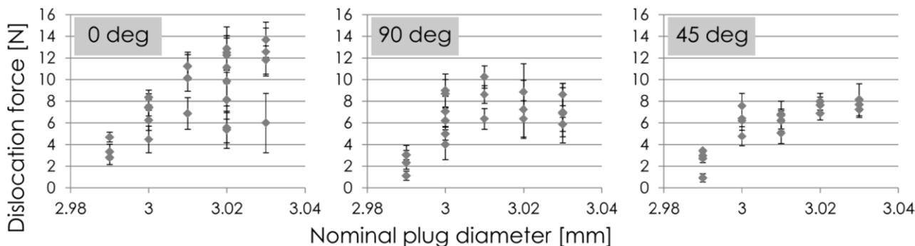
**Figure 5.** Dislocation force normal to the device surface for interconnections fastened with plugs of different sizes. Each point represents the average of eight (0 deg) or four (90 deg and 45 deg) dislocation force measurements for a single plug and a minimum of four plugs were tested for each nominal size. The strength of the interference fit increases with increasing plug size.
