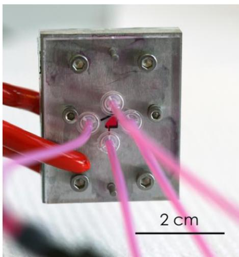
**Figure 7.** The working model of the RheoStream™, a microfluidic flow cell for complex rheology measurements has been interfaced using the interconnection system.
