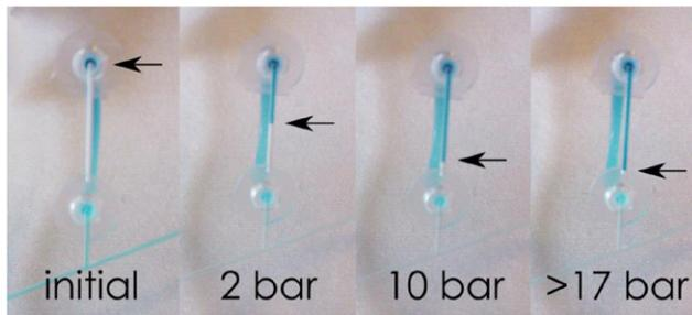
**Figure 4.** Close-up of one of the dead-end channels on the pressure test device. The compression of air in the channel indicates the applied pressure in the system. From this perspective (below the device) leakage can easily be spotted when inspecting the interconnection.
