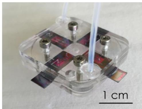
**Figure 6.** Flow cell to interface four silicon sensor chips in two separate flow streams, two sockets for in- / outlet can be seen in the front and back corner of the device. A PDMS sheet with channels in between the PMMA layers forms the sealing interface with the devices.
