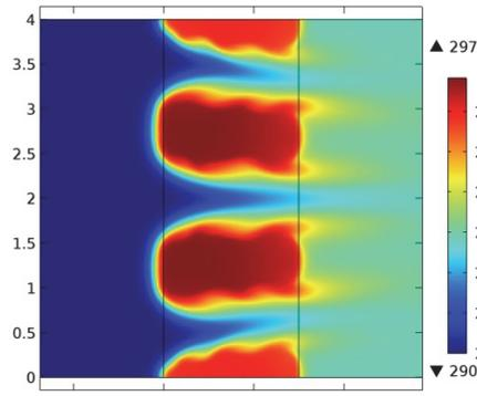
**Figure 4.** Temperature distribution (K) for optimized heat sink.
