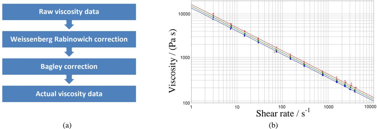
**FIGURE 1.** (a) Flow diagram of viscosity correction process; (b) viscosity curves for the metallic feedstock resulting from the measurements with subsequent corrections.
