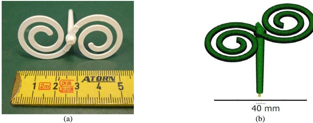
FIGURE 2. (a) Molded spiral test geometry; (b) meshed 3D simulation model of the investigated test spiral with sprue.
