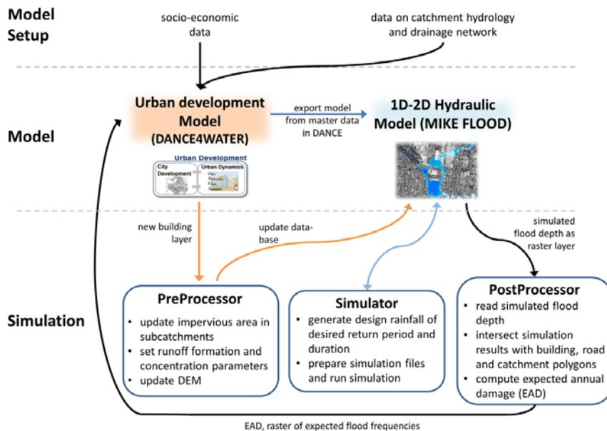
**Figure 1.** Schematic Layout of the integrated simulation tool.
