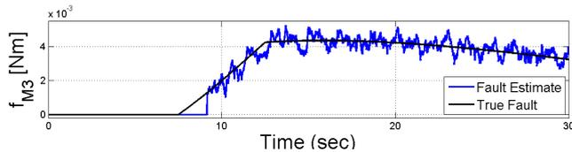
Fig. 7. Estimate of the actuator fault  $F_{M_3}$ .
