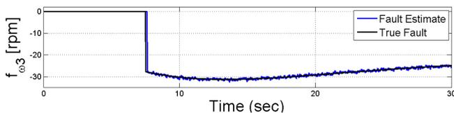
Fig. 8. Estimate of the physical sensor fault  $F_{\omega_3}$ .
