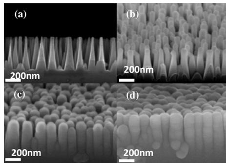
Fig. 1. (a) The SEM cross-sectional image of nano-textured sample. Tilted SEM view of f-SiC nano-textured surfaces deposited with (b) 20nm  $\text{Al}_2\text{O}_3$ , (c) 50nm  $\text{Al}_2\text{O}_3$ , (d) 80nm  $\text{Al}_2\text{O}_3$  film.
