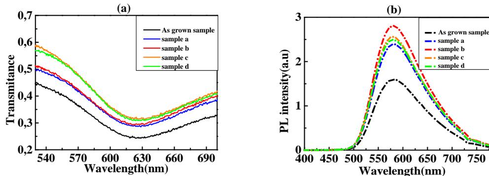
Fig. 2. (a) The optical transmittance curves measured in wavelength range of 520 to 700 nm and (b) photoluminescence spectra for the samples with different thickness of  $\text{Al}_2\text{O}_3$  passivation films.
