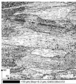
Fig. 2. Boundary map of tungsten warm-rolled to 90% thickness reduction (as-received condition) obtained by EBSD with step size 0.2 μm of an area 224×231 μm<sup>2</sup> on a transversal section containing the rolling and the normal direction, RD and ND, respectively. Grey and black lines represent low and high angle boundaries, respectively.
