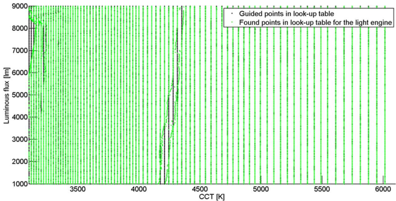
Figure 1: Pre-calibrated lookup table consists of target CCTs (3000 K to 6000 K in 1% step size of the previous CCT and corresponding target luminous flux (1000 lm to 8000 lm in 3% step size of the previous  $\Phi_V$ ) at optimized  $D_{uv}$  ( $< 2 \times 10^{-3}$ ).
