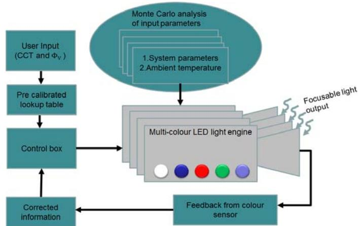
Figure 4: Block diagram of color control system.
