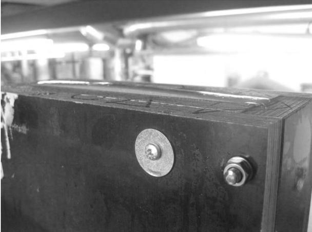
**Fig. 11** Visual assessment of expansion of Mortar C. The photo shows the top of the formwork. After casting Mortar C it was leveled out. During the first 15 min. after casting the mortar raised several mm as can be seen from the photo.
