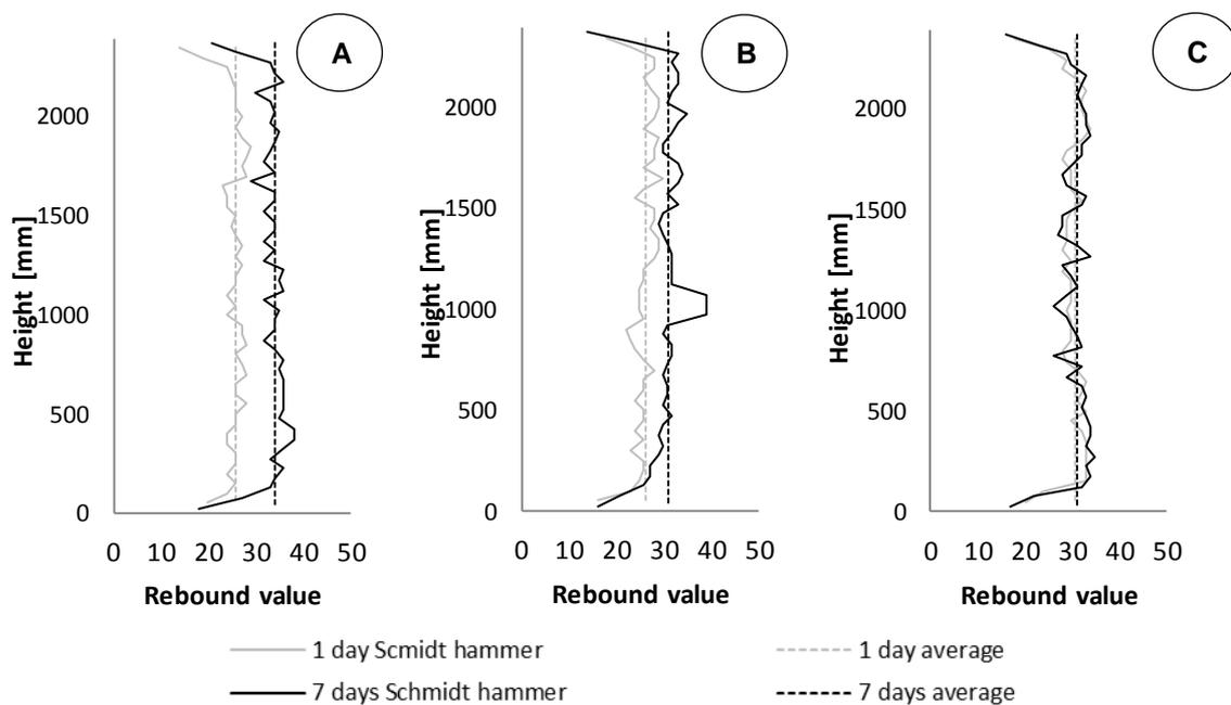
**Fig. 7** Rebound values of Mortar A, Mortar B and Mortar C. The rebound values have been measured after 1 day and 7 days along the height of the mortar joint with a spacing of 5 cm between the measurement points. The rebound values are given without units.
