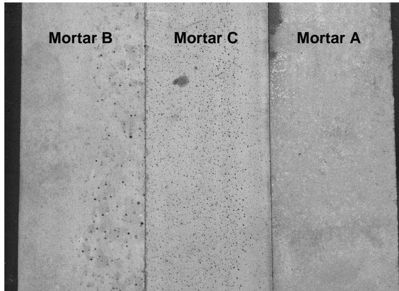
**Fig. 9** Visual appearance of the three mortar surfaces after removing the formwork. The air bubbles in Mortar B were estimated to have an average diameter of 5 mm, whereas they were estimated to have an average diameter of 2 mm for Mortar C, and 0.5 mm for Mortar A. From the photo it can be seen how the air bubbles in Mortar B were mainly located in one side of the mortar joint whereas they were more evenly distributed over the surface of Mortar C. In Mortar A very few air bubbles were seen.
