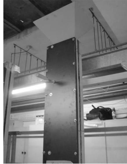
**Fig. 4** The mortar was cast by pouring the mixed mortars through a funnel placed on top of the formwork. Hereby, the mortar had a placing depth of 2400 mm.
