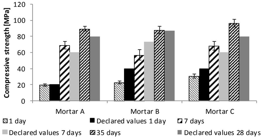
**Fig. 6** 1 day, 7 days and 35 days compressive strengths and standard deviations determined in accordance with EN 196-1 when Mortar A, Mortar B and Mortar C have been mixed in a compulsory mixer. Measured values and declared values are shown. The measured values are based on six specimens each.
