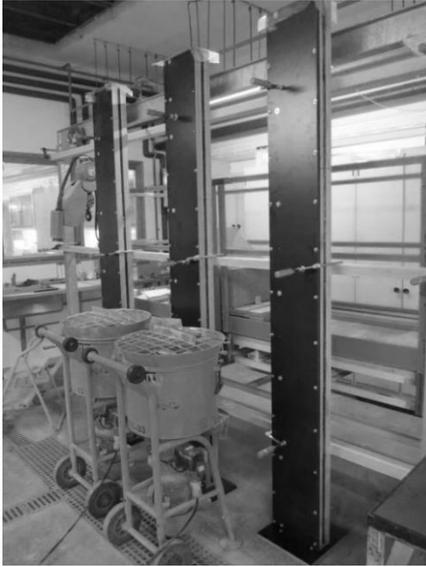
**Fig. 3** Test setup with three wood chambers, each with a dimension of 20 x 220 x 2400 mm. The 40 l compulsory mixers used to mix the mortars are also seen.
