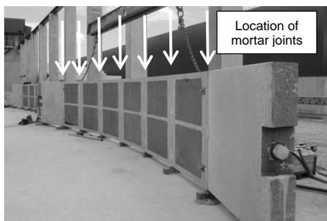
**Fig. 1** Collecting and post-tensioning several SL-Deck Elements to create an arch substructure. The mortar joints between the elements are 1.75 m high. The photo shows a test arch with a span length of 13 m.
