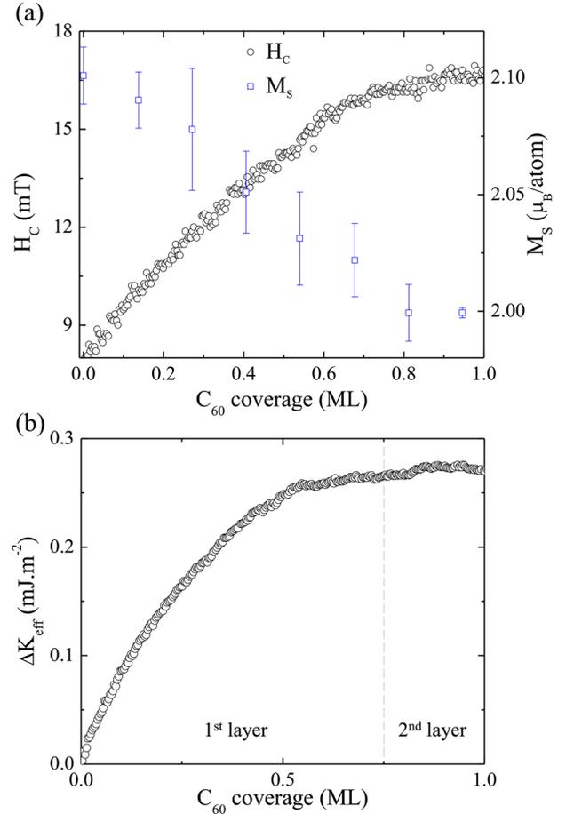
FIG. 2 (color online). (a) Variation of  $H_C$  and  $M_S$  as a function of  $C_{60}$  coverage for a 3.2 ML Co film. (b) Interfacial magnetic anisotropy variation with  $C_{60}$  coverage for a 6.4 ML Co film.
