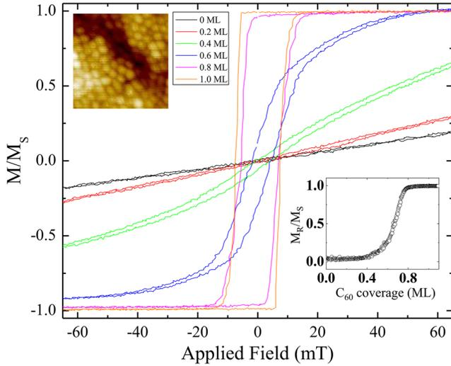
FIG. 1 (color online). Raw hysteresis cycles measured during the deposition of  $C_{60}$  on 5.5 ML Co/Au(111) in a polar MOKE configuration. Bottom inset: Graph of the remanent magnetization  $M_R$  over the saturated magnetization  $M_S$  as a function of the  $C_{60}$  thickness. Top inset: Typical STM image after the deposition of 1 ML of  $C_{60}$  on 5.5 ML Co/Au(111) ( $12 \times 12 \text{ nm}^2$ , 1.0 V, 20 pA).
