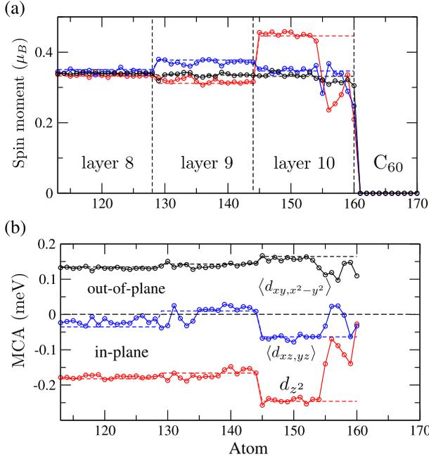
FIG. 4 (color online).  $d$  orbital decomposition of (a) atomic spin moments and (b) MCA for the 10 layers Co slab, pure (dashed lines) and covered with  $C_{60}$  molecules (solid lines). The results for three Co layers close to  $C_{60}$  molecules are only presented. Because of symmetry, contributions from different orbitals in  $\{d_{xz,yz}\}$  and  $\{d_{xy,x^2-y^2}\}$  pairs are very similar so that their averaged values are presented for simplicity.
