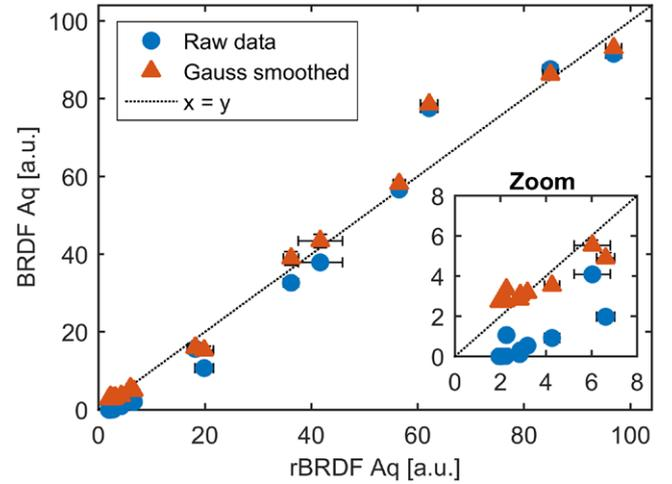
**Figure 6.** Comparison of Aq values obtained from the BRDF and rBRDF instruments. A strong correlation between the values is seen, but only after applying the Gaussian smoothing and the frequency filter of  $f_{\text{max}} = 0.4\mu\text{m}^{-1}$ . Error bars represent  $\pm 1$  SEM on the x values, and  $\pm 1$  SU on the y values.
