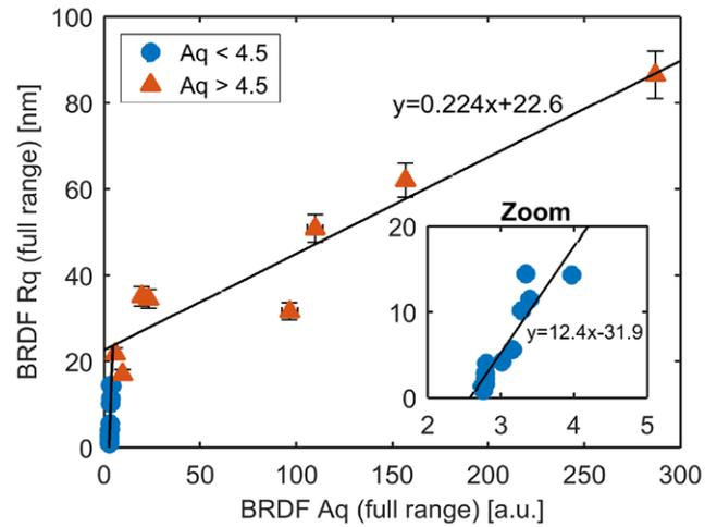
**Figure 8.** Comparison of Rq and  $Aq_{80deg}$  values obtained from the BRDF measurements, showing two regimes of linear correlation, fitted using least squares. Error bars represent  $\pm 1$  SU on both  $x$  and  $y$  values.
