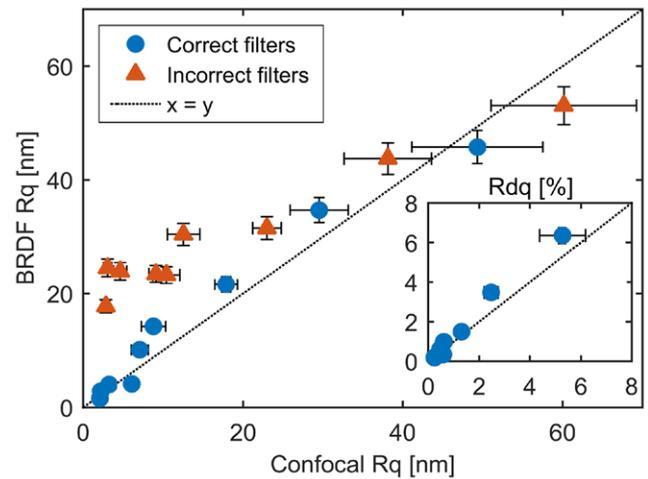
**Figure 4.** Comparison of Rq obtained from the BRDF and confocal instruments, with the corresponding Rdq comparison shown in the insert. One-to-one correlations between the instruments are seen, but only with correct filtering. For this comparison, a subset of only 9 samples was used. Error bars represent  $\pm 1$  SEM on the  $x$  values, and  $\pm 1$  standard uncertainty (SU) on the  $y$  values.
