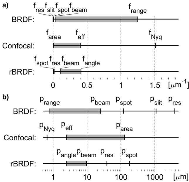
**Figure 2.** Comparison of the frequency limits of the three instruments, (a) in spatial frequency unit, and (b) in spatial wavelengths. The gray rectangles show the resulting bandwidth for each instrument. Note the log scale in (b).
