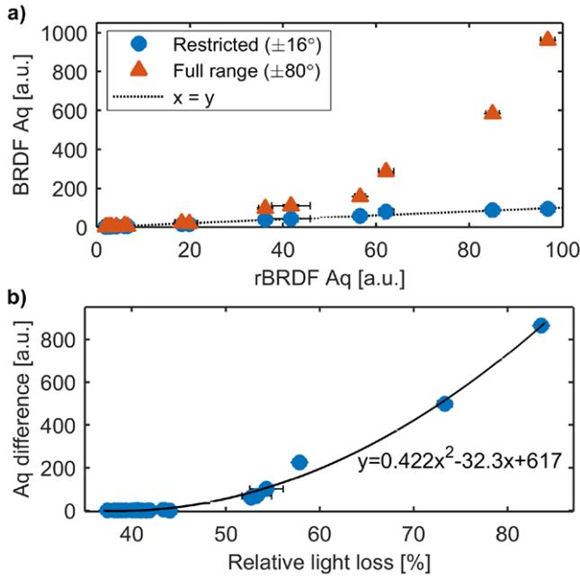
**Figure 7.** (a) Relation between the  $Aq_{rBRDF}$ ,  $Aq_{16deg}$ , and  $Aq_{80deg}$  values. (b) Comparison of the difference in Aq value ( $Aq_{80deg} - Aq_{16deg}$ ) with the relative intensity of light lost outside the restricted range. The lowest loss is not zero because the reflectance of the steel is only  $\sim 67\%$ . Error bars represent  $\pm 1$  SEM on the  $x$  values, and  $\pm 1$  SU on the  $y$  values.
