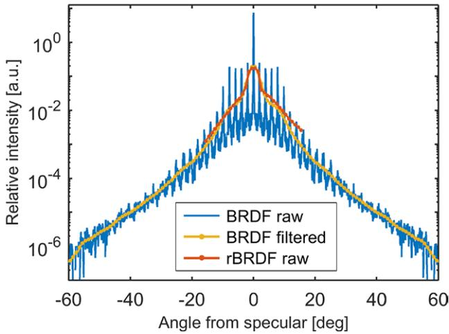
**Figure 5.** Scattering spectra obtained by BRDF and rBRDF instruments. The distinct spikes on the raw BRDF spectrum are caused by a periodic surface feature of  $20\mu\text{m}$ , resulting from the polishing process. The spectra are scaled relative to the area under each curve, and the BRDF spectra shown before cropping.
