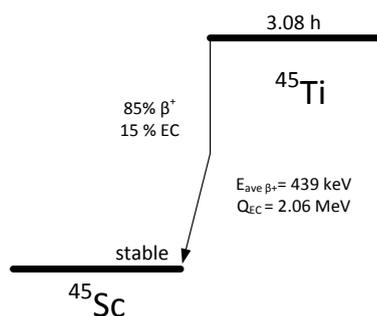
FIGURE 1: The simplified decay scheme of  $^{45}\text{Ti}$
