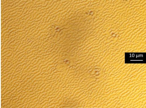
FIG. 2: Precipitated Si clusters on the surface of sample 6 (DIC microscopy)
