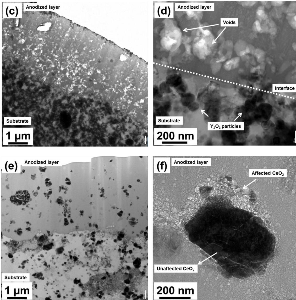
Figure 4: TEM bright field image showing anodized layer cross section of FSP and anodized samples with (a), (b)  $\text{TiO}_2$ , 19 V, (c), (d)  $\text{Y}_2\text{O}_3$ , 10 V and (e), (f)  $\text{CeO}_2$  10 V.
