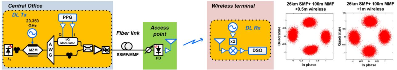
Figure 1. Experimental setup for a W-band fiber-wireless link.
