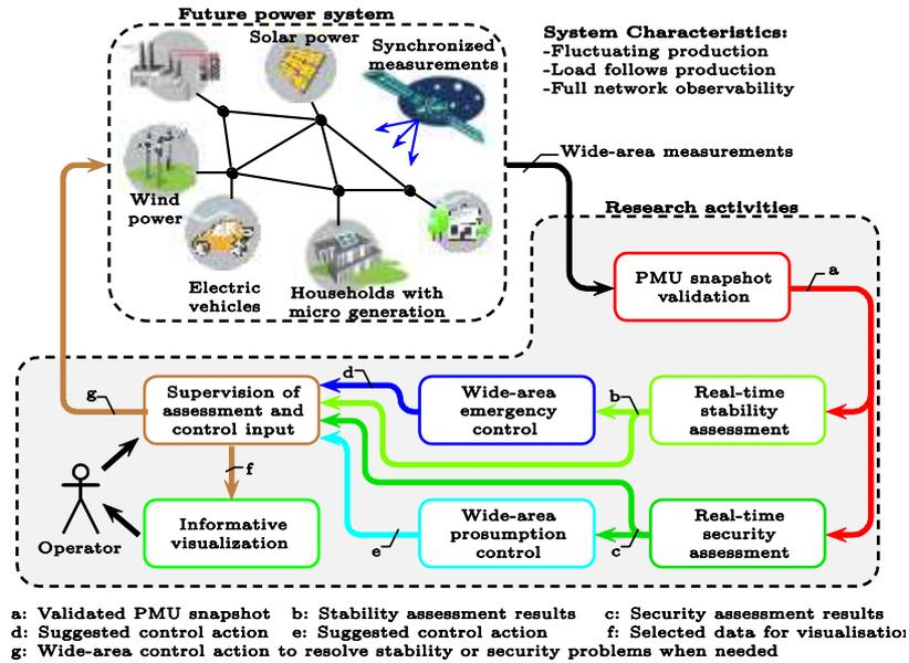
**Fig 1: Conceptual overview illustrating main research activities in the SOSPO project and how the research results contribute to an overall approach for ensuring secure operation of future power systems.**
