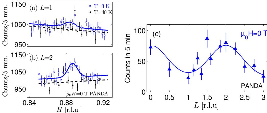
FIG. 5. (color online) (a-b) Scans through ( $H$   $0.14H$   $L$ ) at  $T = 3$  K (blue open squares) and  $T = 40$  K (black points) in zero field for  $L = 1$  (a) and  $L = 2$  (b). (c)  $L$ -dependence of the incommensurate magnetic signal above background in zero field measured at PANDA.
