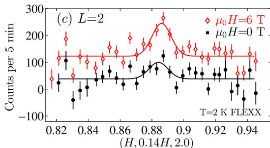
FIG. 3. (color online) Measured peak intensity at  $T = 2$  K for the IC position  $(H, 0.14H, 2.0)$  in 6 T field (red curve) and zero field (black curve). Point-wise background subtraction has been performed, using 40 K data as background. This data was taken at FLEXX, HZB. The field data is shifted upwards by a constant offset for clarity.
