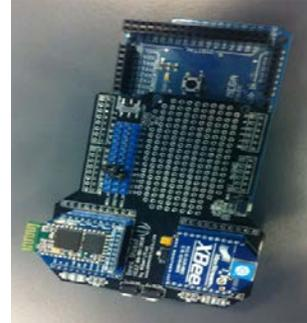
Figure 2. Arduino Uno with beeshielded Bluetooth and Xbee.
