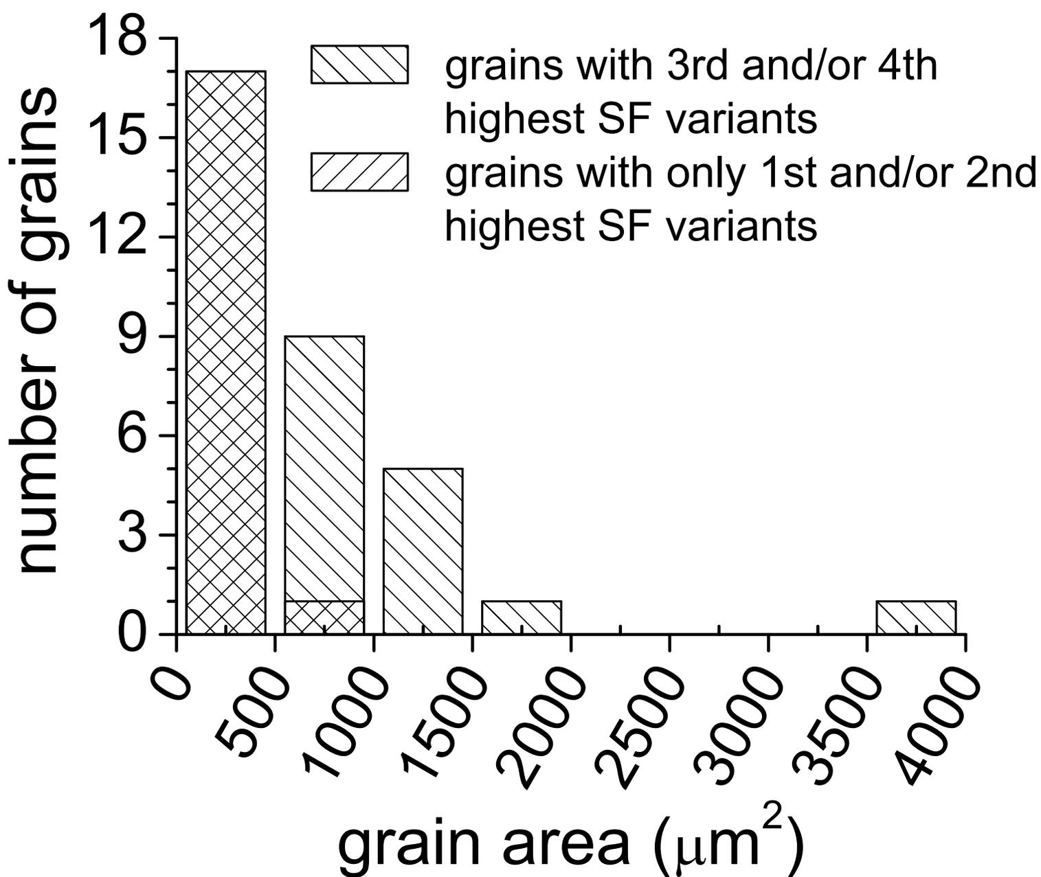
Figure 11: Distribution of grain area for all the grains with compression axis directions corresponding to an  $\alpha$  value  $>0.6$ , where  $\alpha$  is the ratio of the fourth ranked SF to the first ranked SF.
