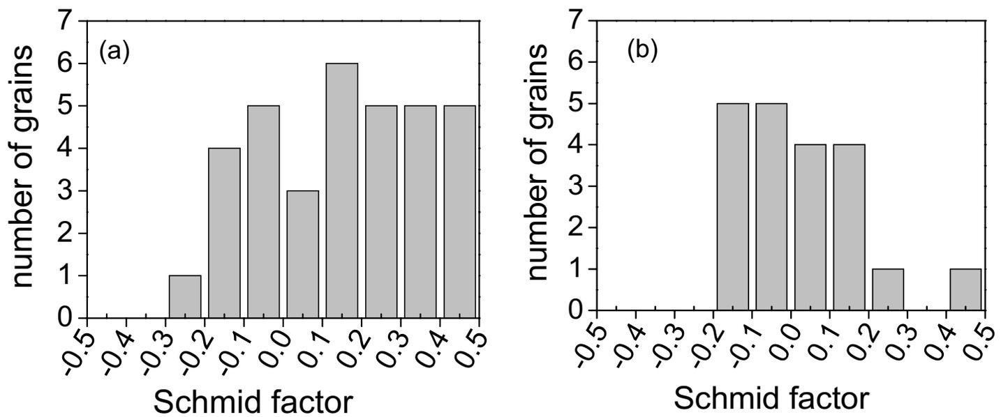
Figure 8: The maximum Schmid factor for untwined grains after compression at 150°C to strains of: (a) 5%; (b) 10%.
