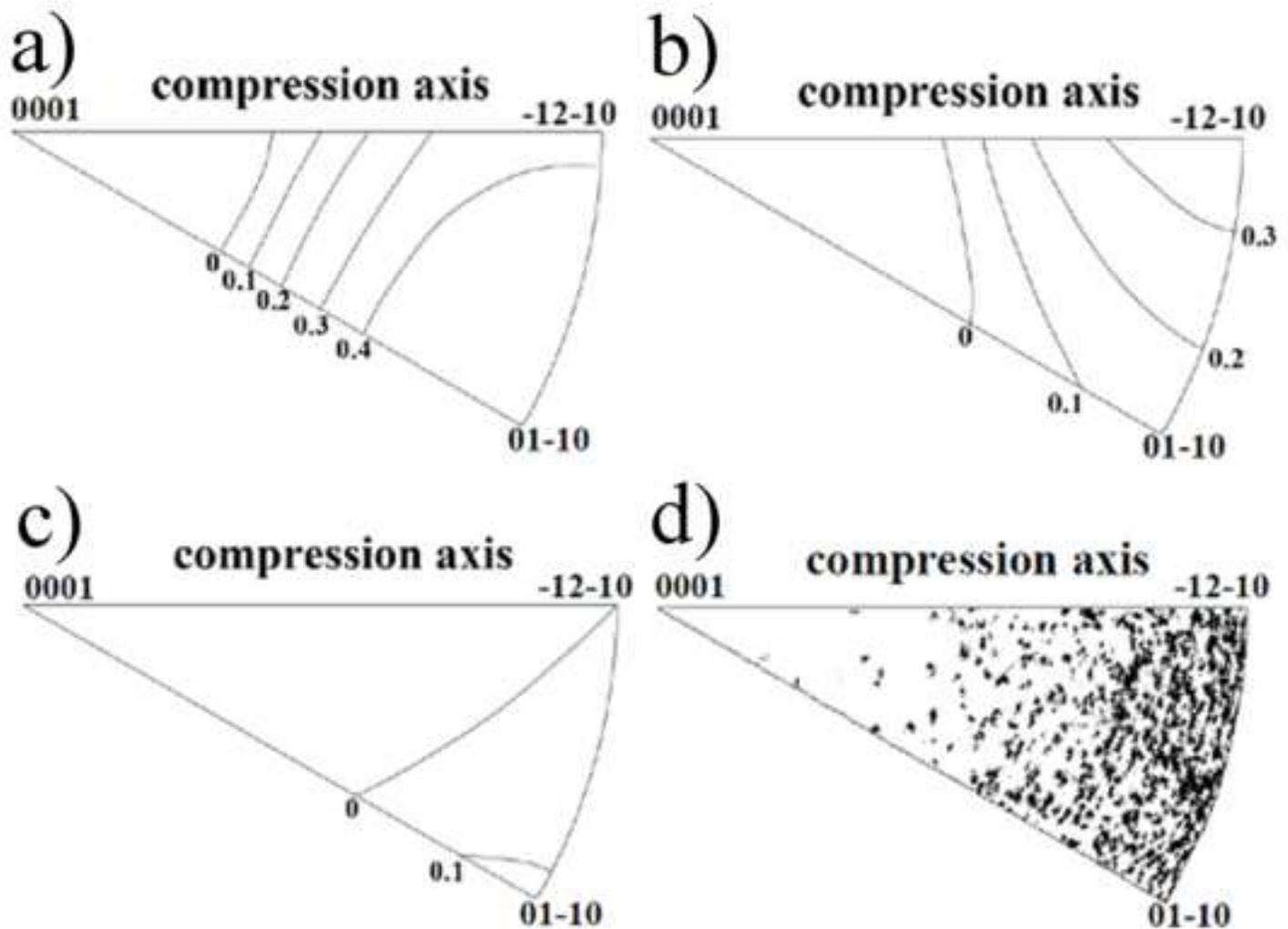
Figure10: Inverse pole figures (compression axis direction) showing contour plots of the variation in Schmid factor (SF) value for the: (a) highest SF, (b) fourth highest SF, (c) sixth highest SF; (d) the orientations of grains for a sample of the initial material used in this study.
