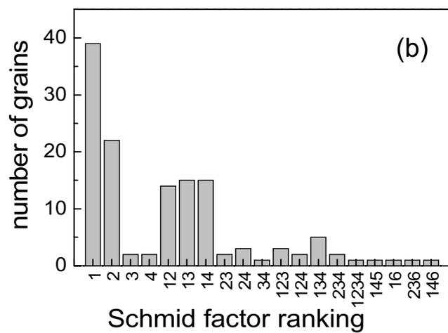
Figure 5: Ranking of Schmid factors for twin variants in samples deformed to strain of (a) 5%, (b) 10% . Example of labelling: Rank "1" represents a grain with a single twin variant with the highest SF; Rank "14" denotes a grain with two twin variants corresponding to the first and fourth highest Schmid factors
