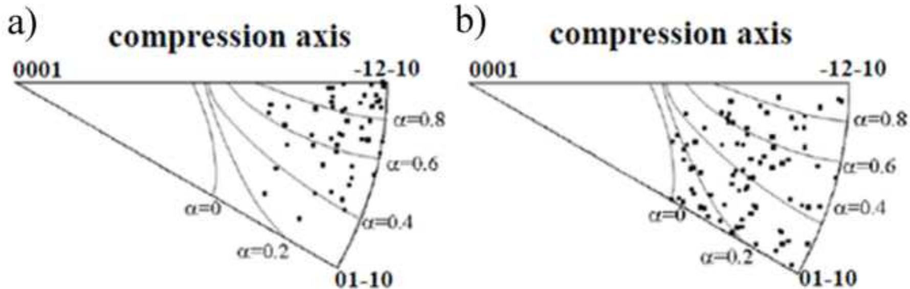
Figure 9: Distribution of grain orientations after 10% deformation for : (a) grains containing twinning variants with third and/or fourth highest Schmid factor (SF); (b) grains only containing twinning variants with first and/or second highest SF. Contours of the ratio of fourth ranked SF to first ranked SF are also shown.
