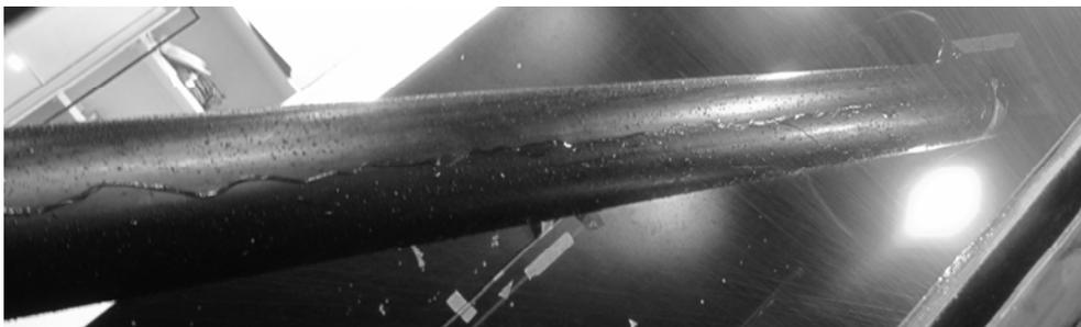
Figure 2. Full-scale yawed cable model (wet tests).
