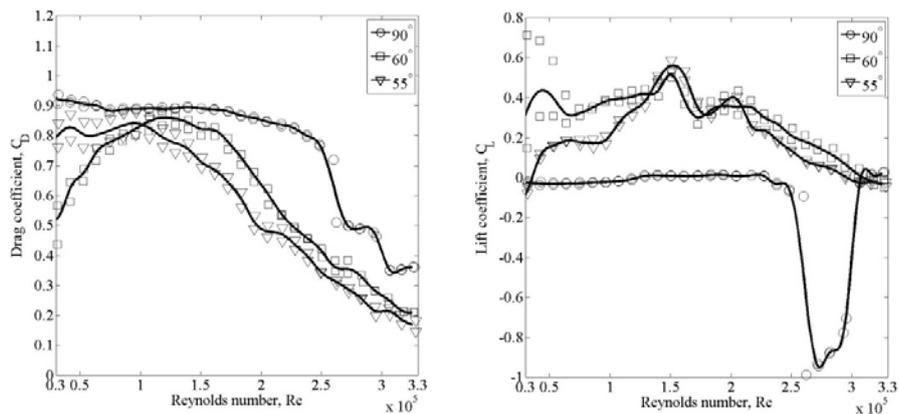
Figure 5. Drag and lift coefficient components for yawed cable model (dry conditions, no end plates).
