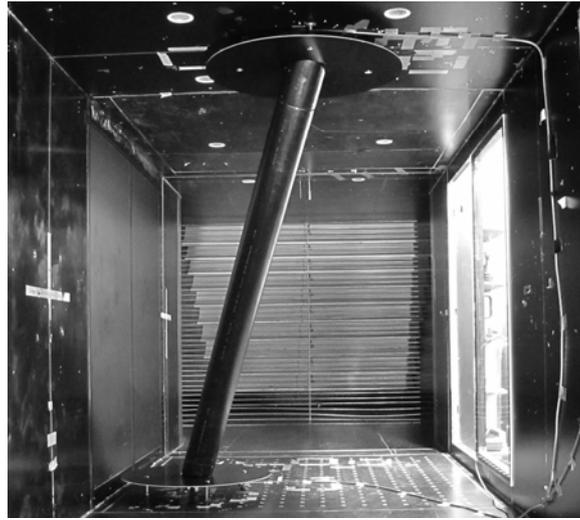
Figure 1. Full-scale, yawed cable model (dry tests).
