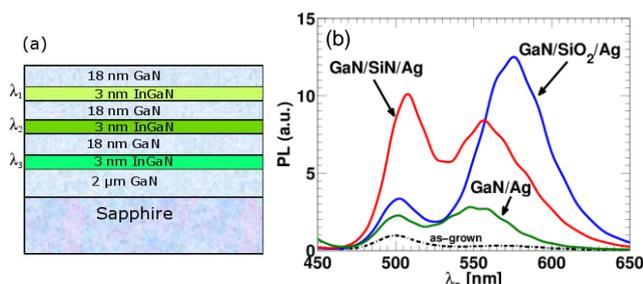
Fig. 1. a) The multiple-color InGaN/GaN QW structure where  $\lambda_1 > \lambda_2 > \lambda_3$ . b) Total PL spectra of the as-grown QW (black dashed). Comparison is made between 20 nm SiO<sub>2</sub> and SiN thin film together with Ag NP coating.
