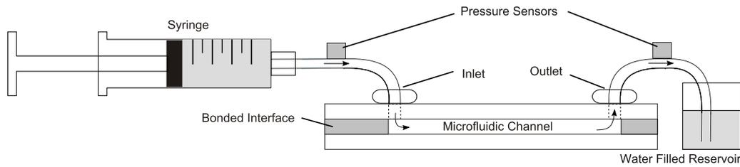
**Figure 3.** Schematic diagram of the setup used to perform pressure drop measurements.
