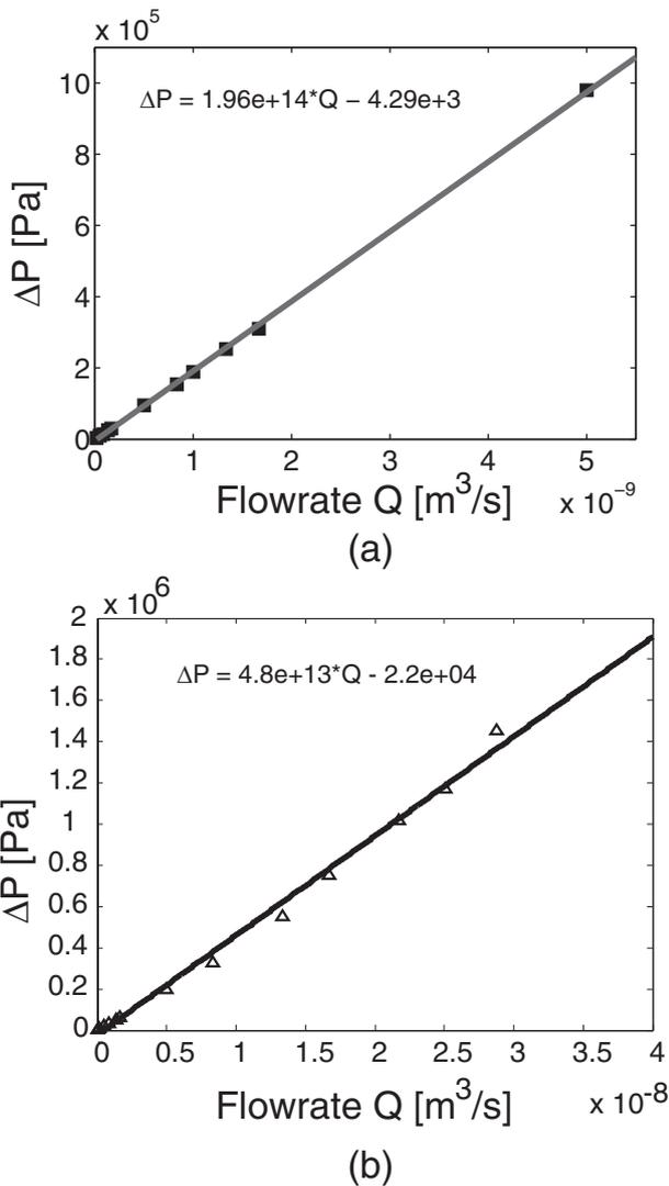
Figure 9. Pressure drop test after bonding (a) PI-PI bonded microfluidic channel with dimensions Length x Width x Height = 3118 x 77 x 22.9 μm (b) PI-glass bonded microfluidic channel with dimensions Length x Width x Height = 3118 x 77 x 11.6 μm.
