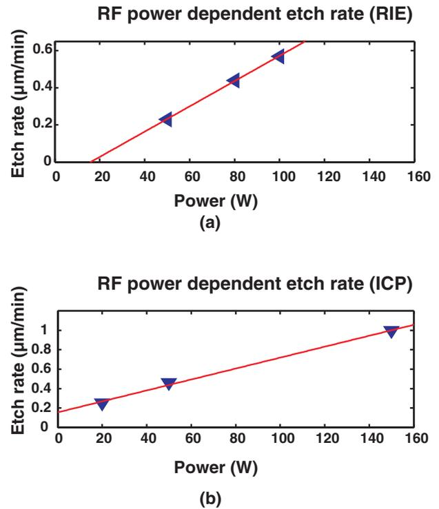
**Figure 4.** Etch rate of partially cured PI as a function of power in the chamber using  $\text{Si}_3\text{N}_4$  mask. (a) In RIE the pressure of the chamber is 200 mTorr and the ratio of  $\text{O}_2/\text{Ar}$  is 98/2 (b) In ICP the pressure of the chamber is 80 mTorr, the ratio of  $\text{O}_2/\text{Ar}$  is 98/2 and Coil power is 2000 W
