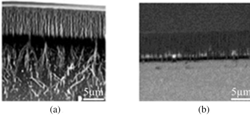
**Figure 5.** SEM images after etching of Polyimide using  $\text{Si}_3\text{N}_4$  mask in RIE (a) Residues are visible if  $\text{CF}_4$  is not used at all for etching PI (b) No residues are visible if the last  $1\ \mu\text{m}$  of PI is etched with mixture of  $\text{O}_2$  and  $\text{CF}_4$ .
