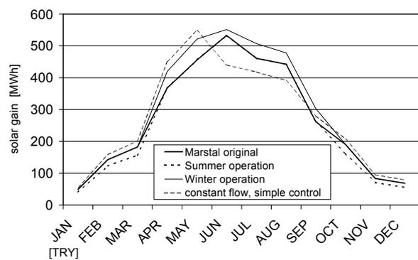
**Figure 1. Comparison of the monthly solar gain for different control strategies and the second generation plant (Marstal case).**
