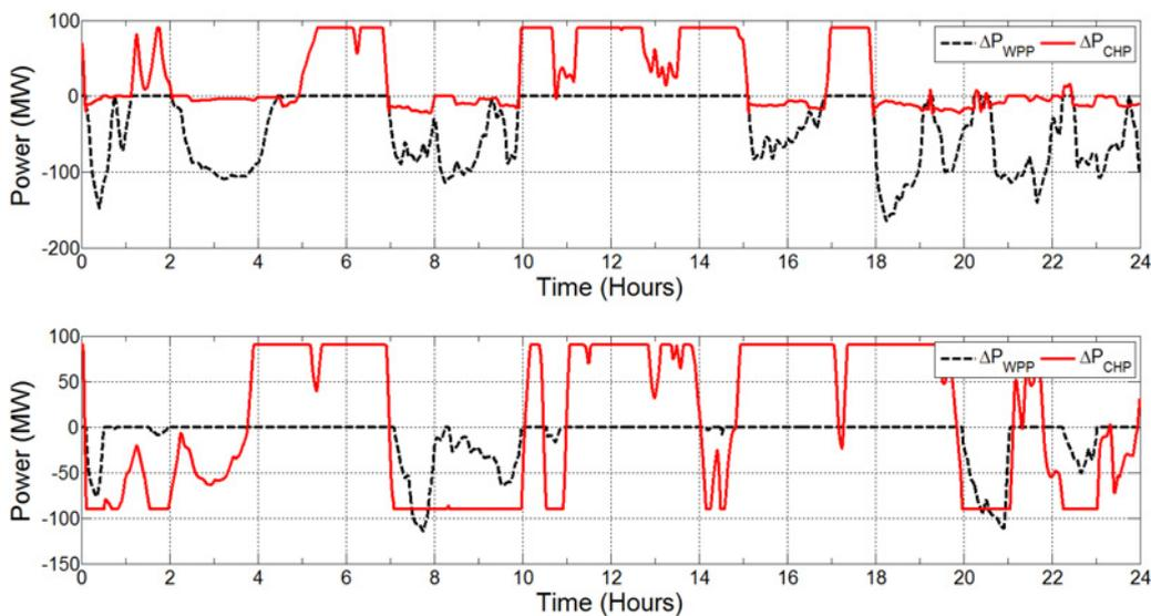
Fig. 9  $\Delta P_{CHP}$  and  $\Delta P_{WPP}$  – top: eastern Danish power system; bottom: western Danish power system
