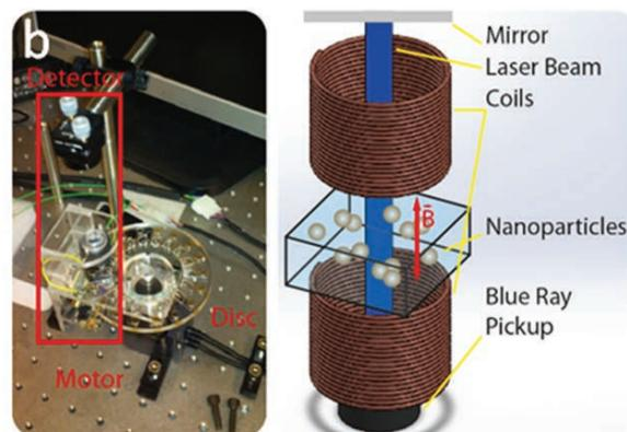
**Figure 2: (a)** Disk for magneto-optical measurements on RCA products **(b)** overall platform comprising a motor, a Sony Blu Ray pickup head, coils for magnetic field excitation and a mirror used to reflect the light back to the photodetector. A customized electronic board is used to extract the signal from the Blu-Ray photodetector.
