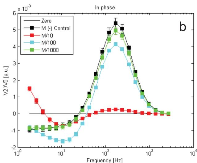
**Figure 3: In phase second harmonic photodetector signals plotted vs. frequency for (a) coils B to the left and (b) monomers M to the right. The coils were measured at 33pM concentration (B/10) and the monomers at 9nM (M/10), 900pM (M/100) and 90pM (M/1000) concentration. The (-) negative control is from a template free C2CA reaction.**
