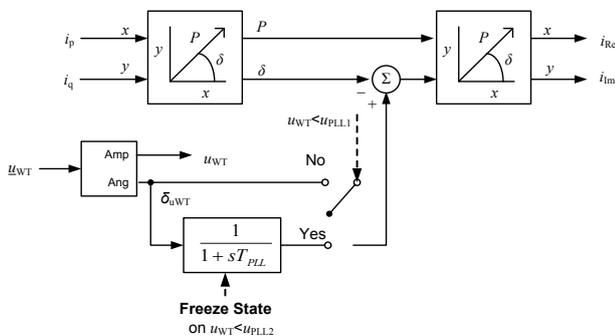
Fig. 2. Block diagram for the reference frame rotation [11]
