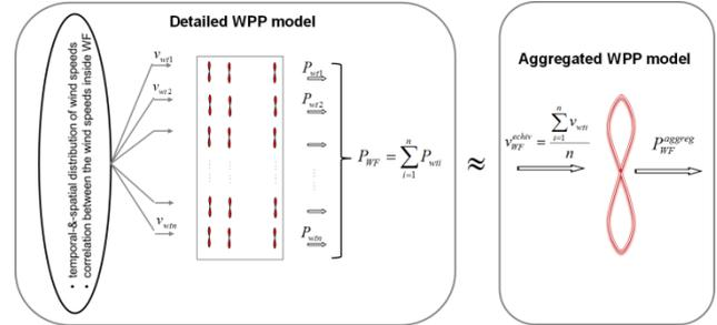
Fig. 6. Wind power plant aggregation method [14]
