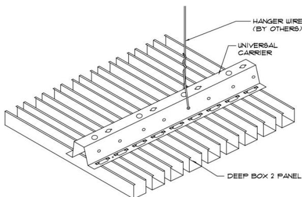
FIG 2. Aluminium lamellas with suspension system
