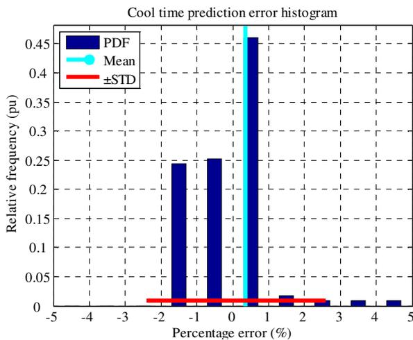
Fig. 10 Histogram of cool cycle time prediction error
