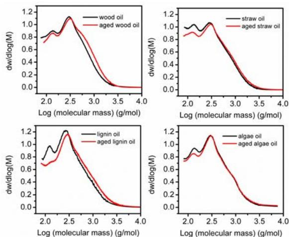
**Figure 5:** The molecular mass distribution of bio-oils
