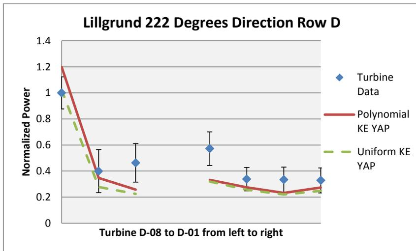
Fig. 6 Power predicted by two different thrust distributions for a resolution of D/8 versus experimental power data retrieved from Lillgrund for  $222 \pm 2.5$  degrees and  $9.0 \pm 0.5$  m/s when using the k-epsilon with YAP correction turbulence closure model.
