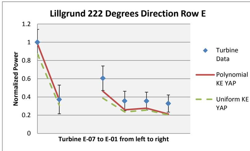
Fig. 7 Power predicted by two different thrust distributions for a resolution of D/8 versus experimental power data retrieved from Lillgrund for  $222 \pm 2.5$  degrees and  $9.0 \pm 0.5$  m/s when using the k-epsilon with YAP correction turbulence closure model.
