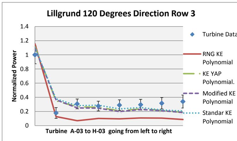
Fig. 8 Power predicted for four different turbulence models for a resolution of D/8 versus experimental power data retrieved from Lillgrund for  $120 \pm 2.5$  degrees and  $9.0 \pm 0.5$  m/s for the polynomial distribution.
