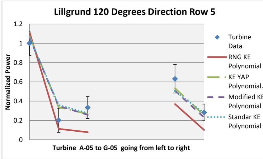
Fig. 9 Power predicted for four different turbulence models for a resolution of  $D/8$  versus experimental power data retrieved from Lillgrund for  $120 \pm 2.5$  degrees and  $9.0 \pm 0.5$  m/s for the polynomial distribution.
