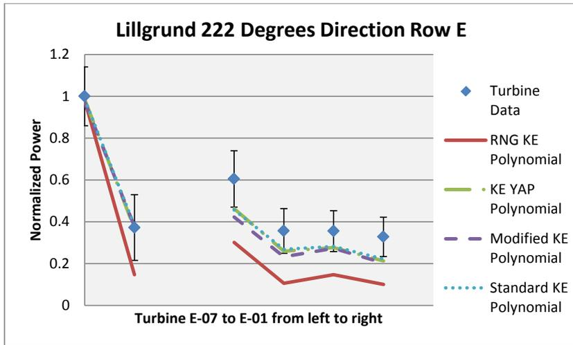
Fig. 12 Power predicted for four different turbulence models for a resolution of  $D/8$  versus experimental power data retrieved from Lillgrund for  $222 \pm 2.5$  degrees and  $9.0 \pm 0.5$  m/s for the polynomial distribution.
