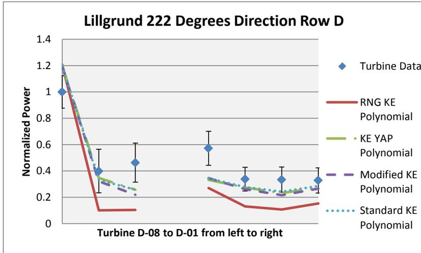
Fig. 11 Power predicted for four different turbulence models for a resolution of  $D/8$  versus experimental power data retrieved from Lillgrund for  $222 \pm 2.5$  degrees and  $9.0 \pm 0.5$  m/s for the polynomial distribution.
