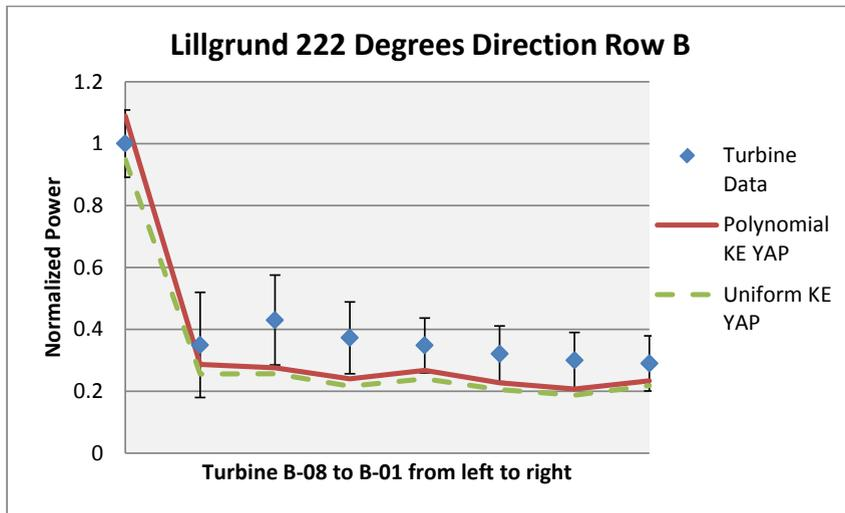
Fig. 5 Power predicted by two different thrust distributions for a resolution of D/8 versus experimental power data retrieved from Lillgrund for  $222 \pm 2.5$  degrees and  $9.0 \pm 0.5$  m/s when using the k-epsilon with YAP correction turbulence closure model.
