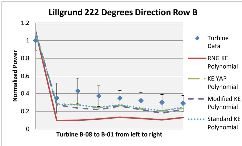
Fig. 10 Power predicted for four different turbulence models for a resolution of  $D/8$  versus experimental power data retrieved from Lillgrund for  $222 \pm 2.5$  degrees and  $9.0 \pm 0.5$  m/s for the polynomial distribution.
