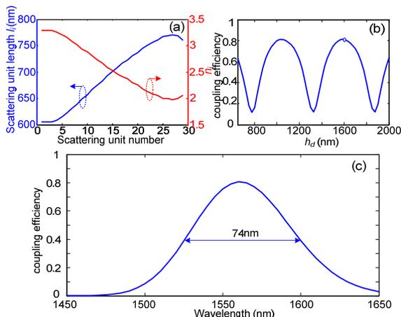
Fig. 2. (a) Designed scattering unit length  $l_s$  and refractive index  $n_s$  distributions of the grating coupler. (b) Simulated coupling efficiency as a function of lower cladding thickness. (c) Simulated coupling efficiency as a function of wavelength with  $h_c=1.6 \mu\text{m}$  and  $h_s=1 \mu\text{m}$ .
