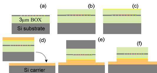
Fig. 3. Fabrication process of the grating coupler with bonded mirror. (a) Grating coupler fabrication based on standard e-beam lithography and ICP etching. (b)  $\text{SiO}_2$  deposition. (c) Metallic mirror deposition. (d) BCB spinning for both sample and carrier wafer. (e) Bonding. (f) Si substrate removal.
