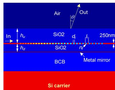
Fig. 1. Schematic structure of the proposed grating coupler.
