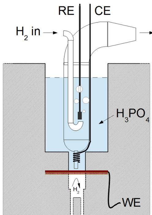
**Figure 2.** Schematic representation of the electrochemical cell used for the HER activity measurements.
