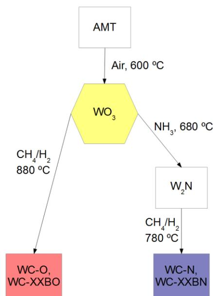
**Figure 1.** Reaction routes used for preparation of WC powders from ammonium metatungstate (AMT). Left: the oxide route where the obtained carbide was named WC-O. Right: the nitride route where the obtained carbide was named WC-N.
