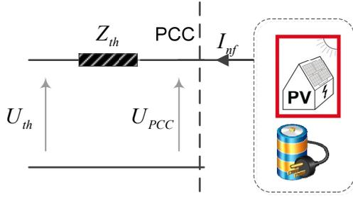
Fig. 1. The thevenin equivalent of a PV system, storage and the local load connected to a typical LV grids.
