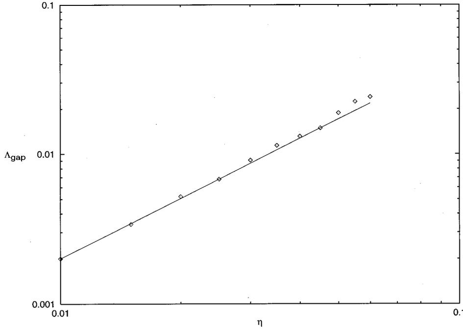
FIG. 3. The width of the gap,  $\Lambda_{\text{gap}}$  vs the disorder strength  $\eta$ . Results of numerical calculations are indicated by squares while the analytical dependence given by Eq. (46) is shown by the solid line. The gap is measured at  $N=0.4$ .
