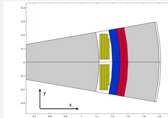
Fig. 3 Simplified model of a synchronous HTS machine with air-gap winding. The magnetic steel is gray, armature winding is dark red, thermal insulation (vacuum chamber, spacers, radiation shields) is blue and space for HTS coils is yellow.
