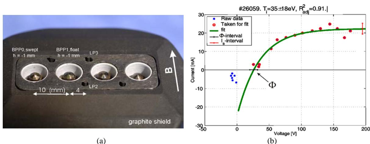
**Figure 1.** a) Quadruple ball-pen probe of AUG. b) Example of  $I$ - $V$  characteristic of swept BPP0 with exponential fit. The red points are used for the fit procedure, the green line shows the resulting fit of the electron branch.
