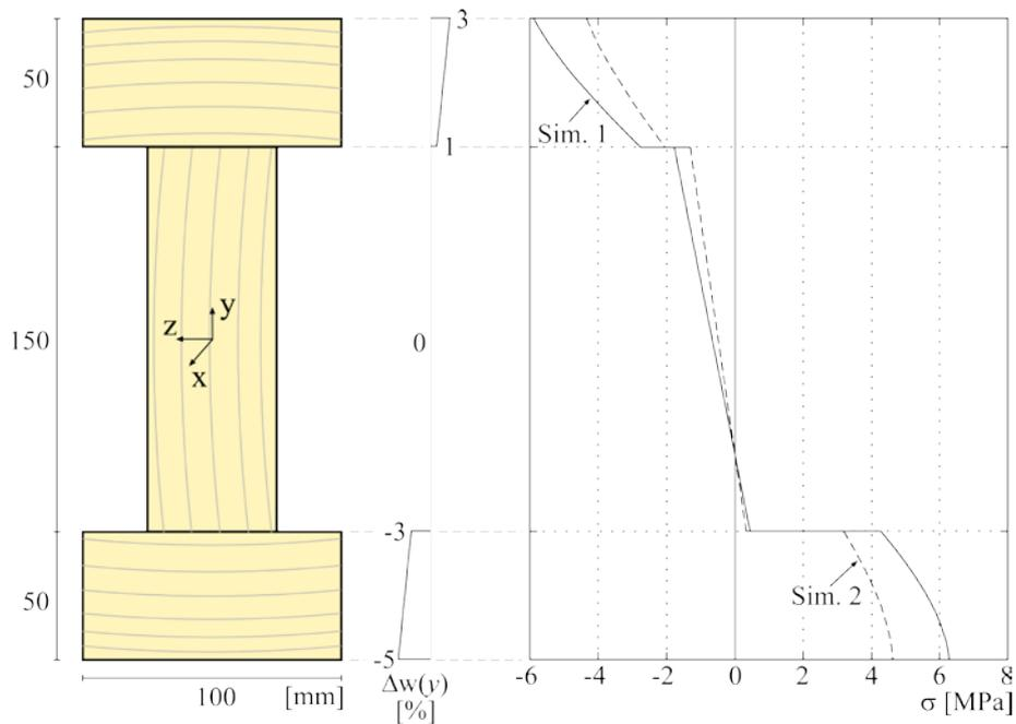
**Figure 5.** Stress distribution in an inhomogeneous two-span I-beam exposed to the same changes in moisture content as shown in Fig. 4, ( $E(y)$  and  $\alpha(z)$  being the same functions as in Fig. 2).
