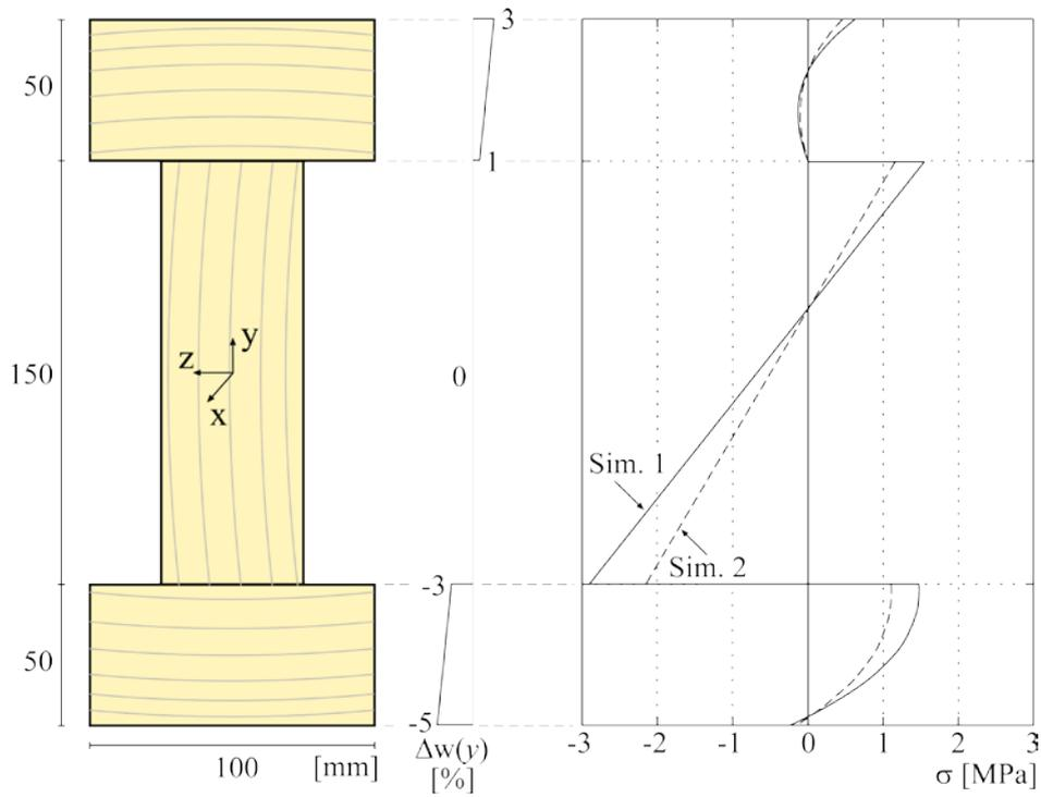
**Figure 4.** Stress distribution in an inhomogeneous simply-supported I-beam exposed to a linearly distributed change in moisture content within the flanges and to no moisture change within the web, ( $E(y)$  and  $\alpha(y)$  being the same functions as in Fig. 2).
