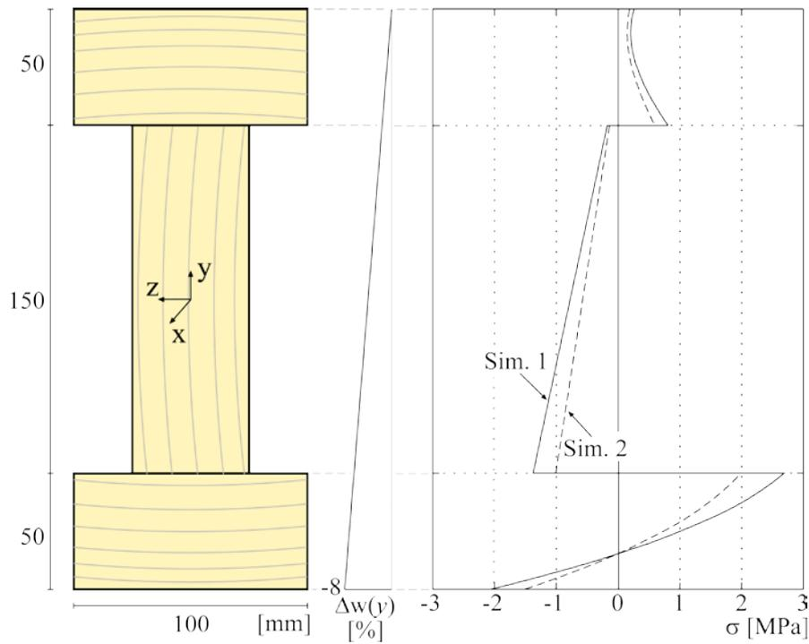
**Figure 3.** Stress distribution in an inhomogeneous simply-supported I-beam exposed to a linearly distributed change in moisture content over the cross section, ( $E(y)$  and  $\alpha(y)$  are the same functions as in Fig. 2).
