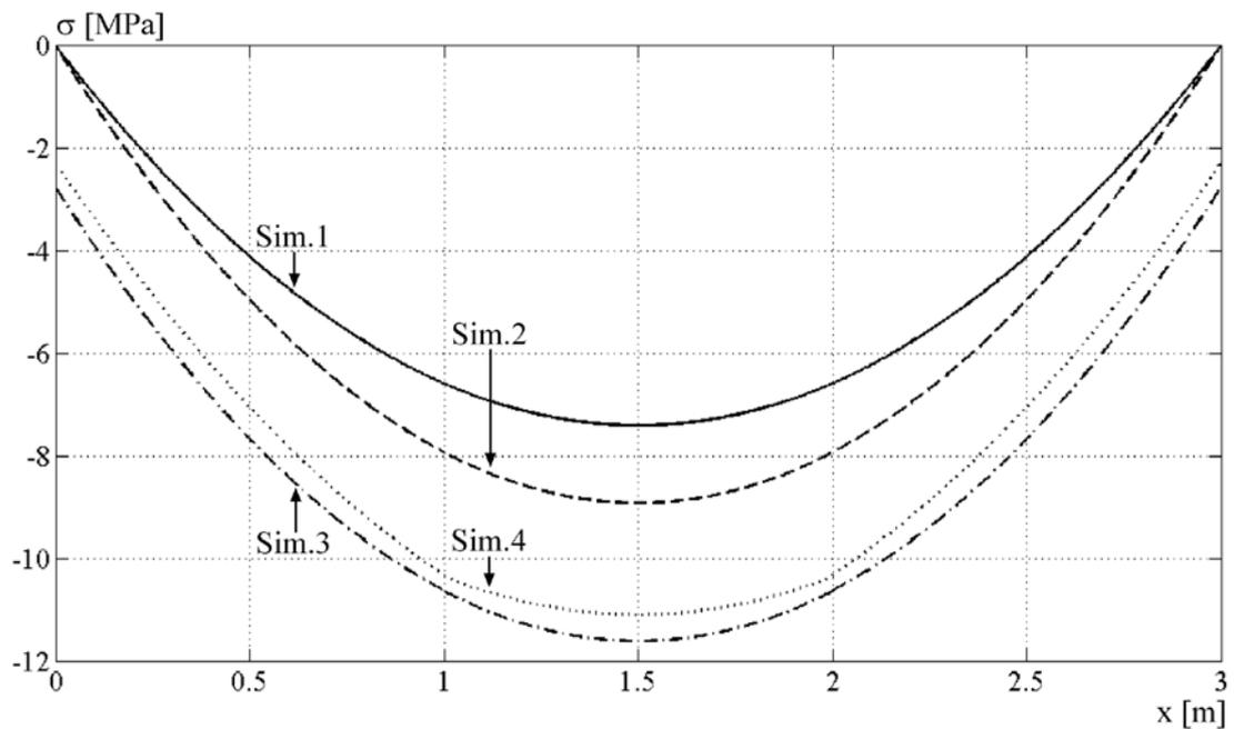
**Figure 10.** Variations in stress along the top surface of the glulam beam shown in Fig. 9.
