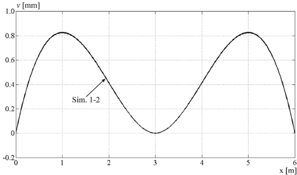
**Figure 8.** Deflection of the continuous I-beam presented in Fig. 5, ( $E(y)$  and  $\alpha(y)$  are the same functions as in Fig. 2).
