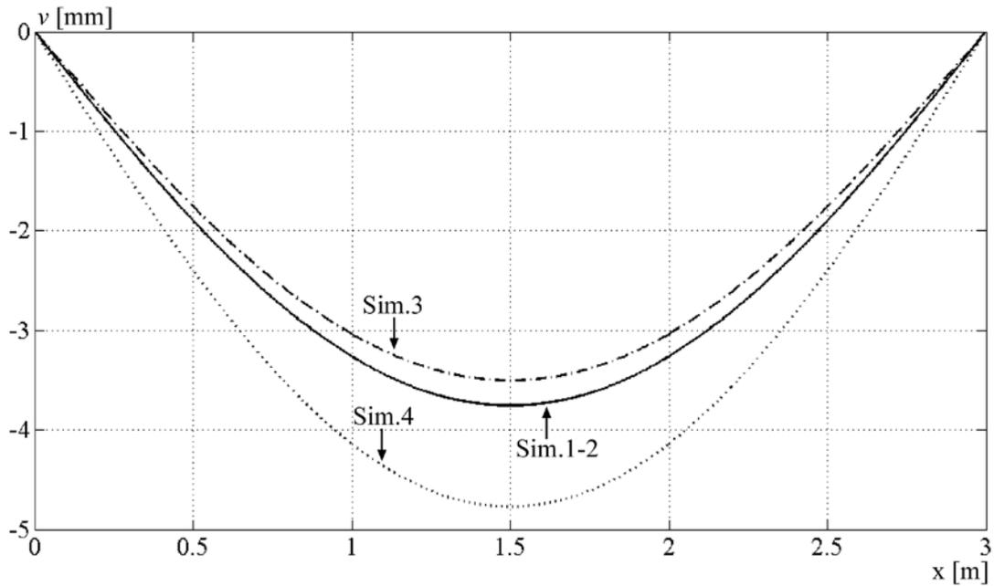
**Figure 11.** Deflection graphs of the glulam beam shown in Fig. 9.
