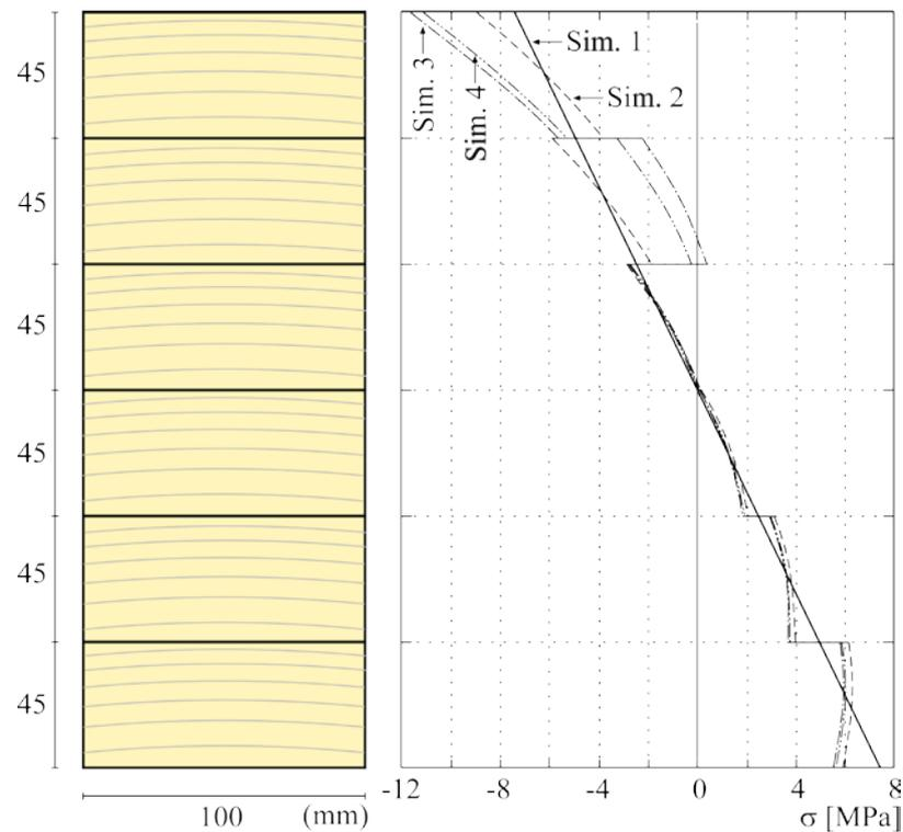
**Figure 9.** Stress distribution in a glulam beam:
