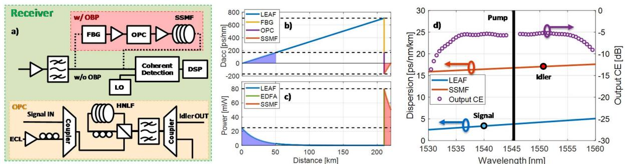
Fig. 1. (a) Schematics of OBP and OPC modules at the receiver. (b) Evolution of accumulated dispersion and (c) power versus distance with OBP module at the receiver included. (d) Dispersion characteristics of LEAF (blue) and SSMF (red) versus wavelength with signal, pump and idler position indicated, and output conversion efficiency of HNLF (purple).
