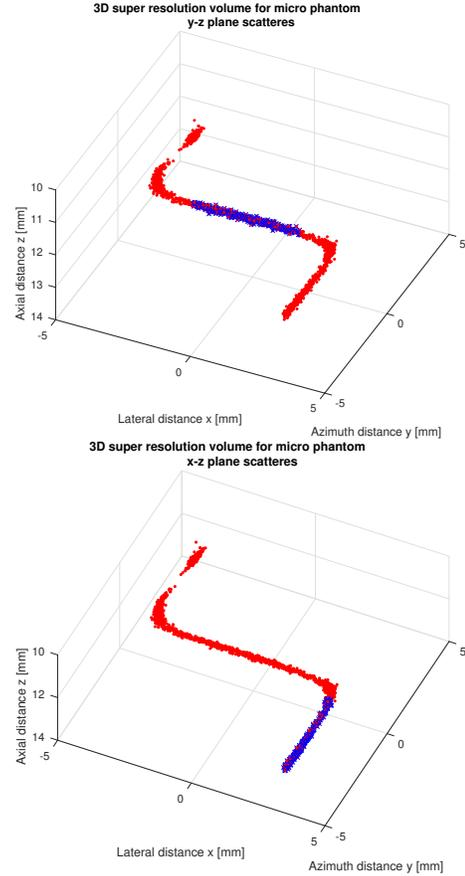
Fig. 2. Identification of bubbles only flowing in the  $x$  direction (top) and only in the  $y$  direction in the outlet (bottom). Red dots show all the bubble locations and blue crosses are the selected bubbles.
