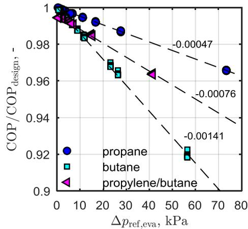
**Figure 2: Normalized COP as a function of total refrigerant pressure drop in the evaporator**
