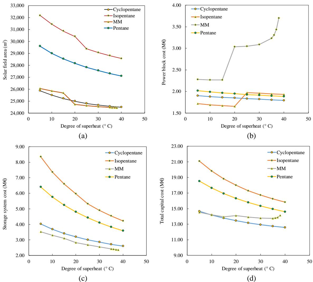
**Figure 2:** Effects of variations in degree of superheat for turbine inlet temperature for current plants on (a) solar collector field area, (b) power block cost, (c) storage system cost, and (d) total capital cost.
