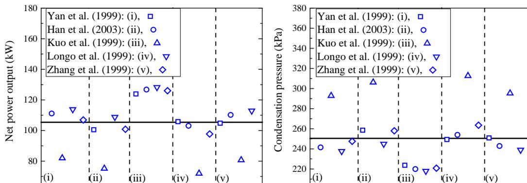
**Figure 4.** Impact of heat transfer correlation on: a) net power output; b) condensation pressure. The solid lines represent the expected design values, the vertical dotted lines separate solutions attained using condensers designed using the various correlations (indicated by roman numbers), and the marker
