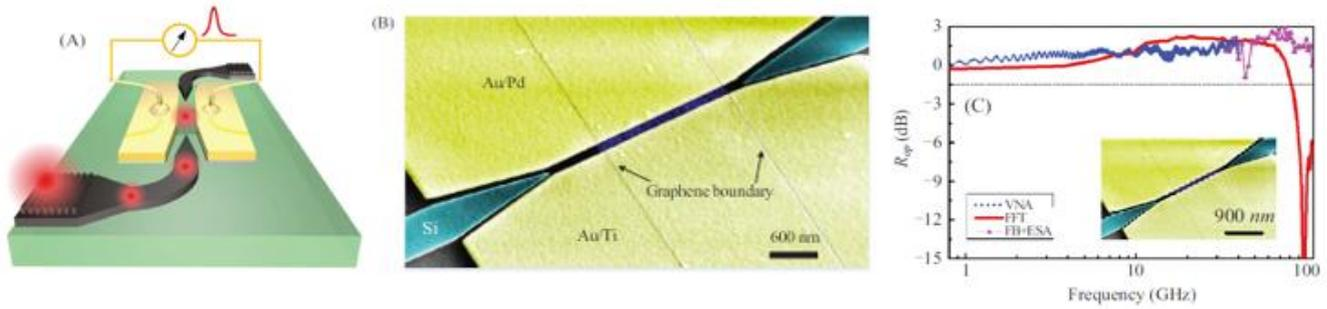
Figure 2. (a) Schematic of the proposed graphene-plasmonic hybrid photodetector (b) An example of fabricated graphene plasmonic photodetector with the graphene coverage length of 2.7  $\mu\text{m}$  (c) Its corresponding optical bandwidth measured by VNA, impulse response, and frequency beating with ESA at the bias voltage of 1.6V.
