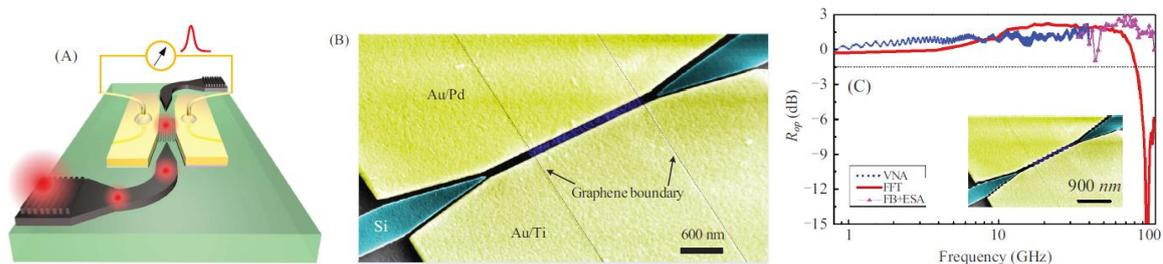
**Fig. 1** (a) Schematic of the proposed graphene-plasmonic hybrid photodetector (b) An example of fabricated graphene plasmonic photodetector with the graphene coverage length of 2.7  $\mu\text{m}$  (c) Its corresponding optical bandwidth measured by VNA, impulse response, and frequency beating with ESA at the bias voltage of 1.6V.
