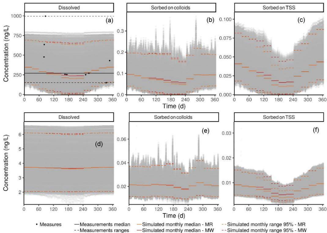
**Figure 2** Predicted concentration (12:00 ranges of (a) diclofenac and (b) triclosan at the outlet of the simulated canal stretch. Measured values were only available for dissolved diclofenac. The simulation started on 1<sup>st</sup> January (day 0) and ended on 31<sup>st</sup> December (day 365).
