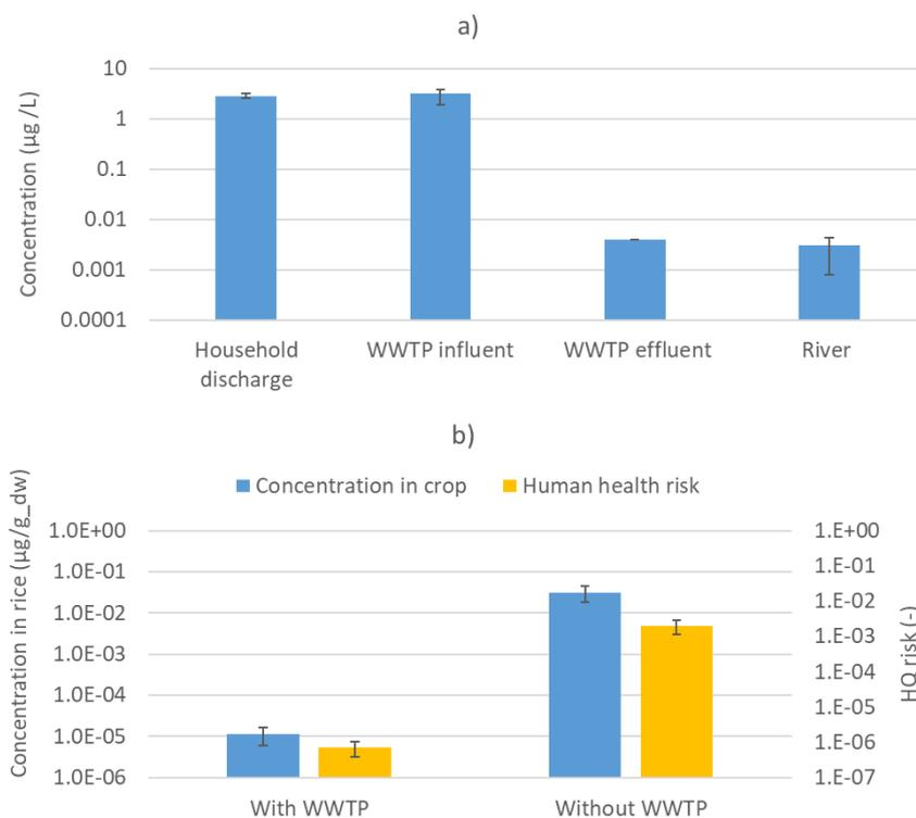
**Figure 3** (a) paracetamol water concentration in different elements of the integrated urban water system, b) paracetamol concentration in rice grains and associated risk (HQ) when irrigation is done with treated and untreated wastewater. Results are expressed as annual means and 5<sup>th</sup>–95<sup>th</sup> percentile ranges.
