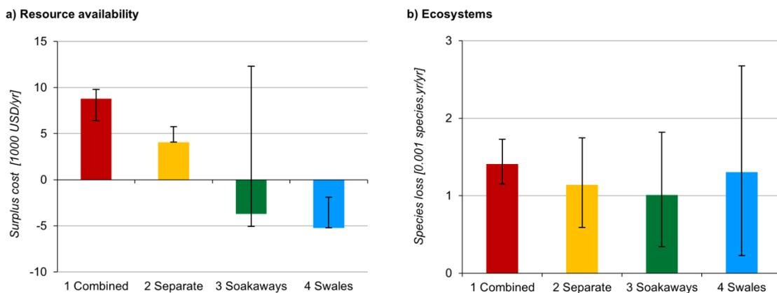
Figure 2. Damage to a) resource availability, b) ecosystems, caused by four different systems managing stormwater according to Danish flood safety and pollution management standards in a catchment area of 260ha. Negative values indicate prevented damages. Error bars illustrate the damages for a worst and best case for each system, varying both infrastructure processes and point source emissions (Brudler et al., 2019a)
