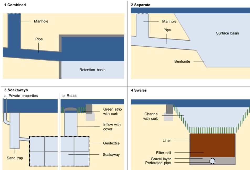
Figure 3. Schematic sketches of the elements in the four different stormwater management systems. The water level during an event with a return period of 5 (10) years is illustrated in light (dark) blue. The water level rises above surface level for events with a return period of 10 years in the systems 2-4 (Brudler et al., 2019a)
