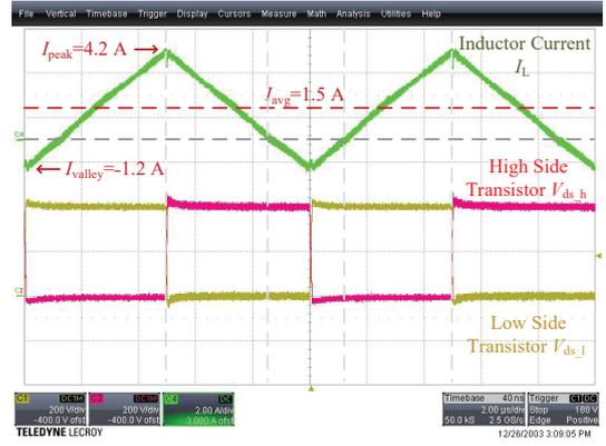
Fig. 8. Experimental waveform of the synchronous buck converter.
