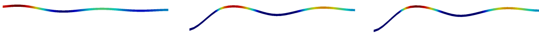
Figure 7. 3500Hz excitation frequency, vibration pattern for the the starting guess (left), optimized design with 1 element in the vertical direction (middle) and optimized design with 5 elements in the vertical direction (right).
