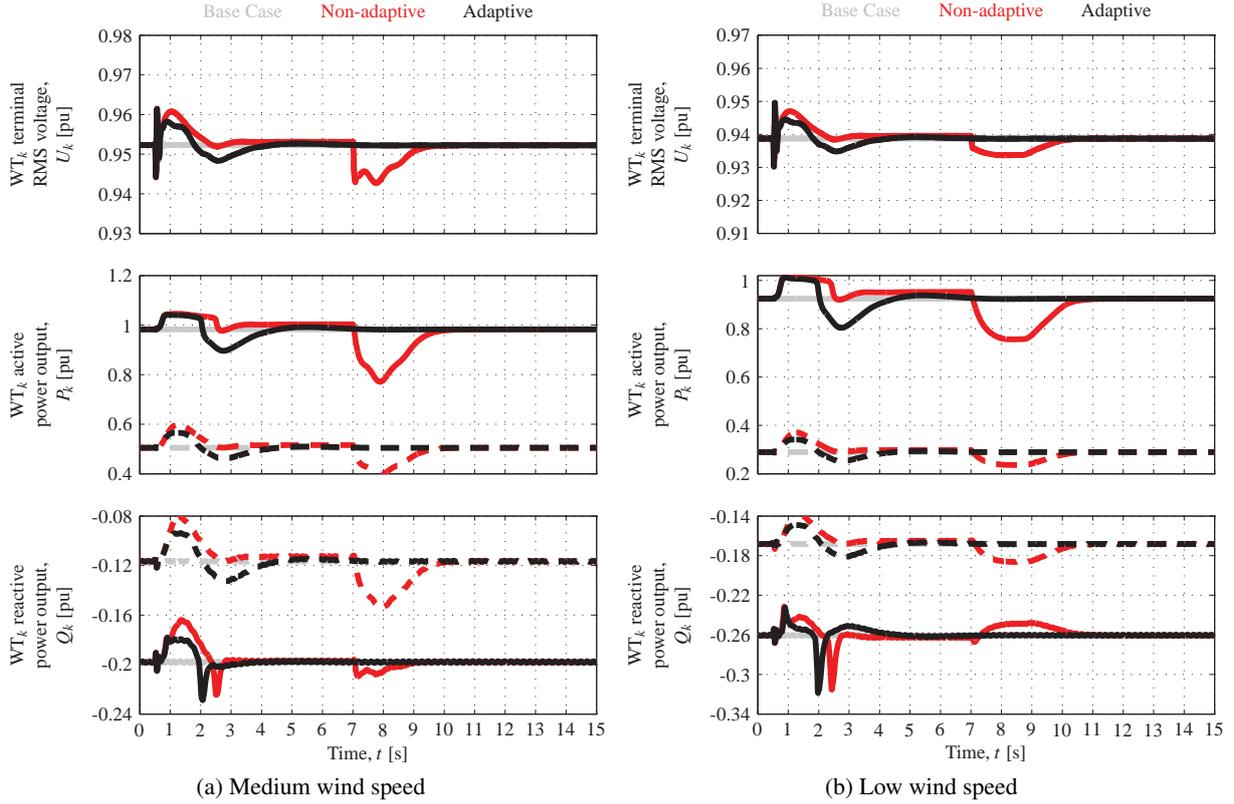
Figure 6:  $k$ th wind turbine response to an onshore underfrequency event – Solid:  $k = 1$ , Dashed:  $k = 9$
