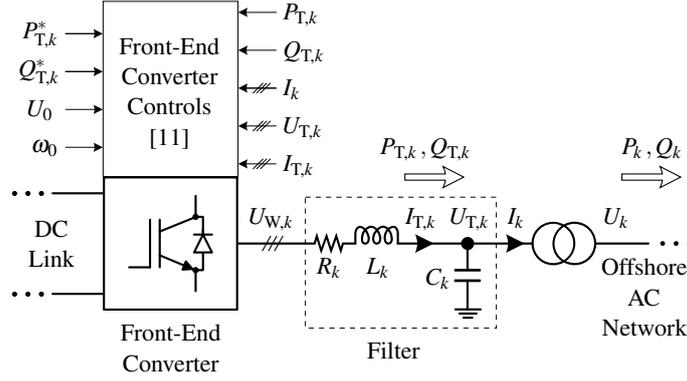
Figure 2:  $k$ th wind turbine front-end (line-side) network
