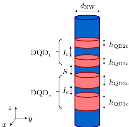
FIG. 5: Two DQDs in a nanowire. The geometrical parameters of  $DQD_c$  are  $h_{QD1c} = 11$  nm,  $h_{QD2c} = 10$  nm,  $I_c = 8$  nm, and the parameters of  $DQD_t$  are  $h_{QD1t} = 5$  nm,  $h_{QD2t} = 3$  nm,  $I_t = 10$  nm. The nanowire diameter is  $d_{NW} = 40$  nm.
