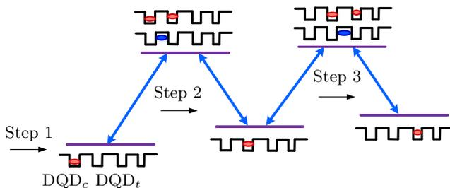
FIG. 13: Scheme for initializing the electrons in a two-DQD. The electron is transferred from QD<sub>1</sub> of DQD<sub>c</sub> to QD<sub>1</sub> of DQD<sub>t</sub> using two STIRAP processes.
