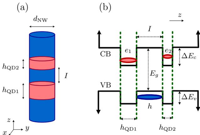
FIG. 1: (a) A DQD in a nanowire. (b) The conduction and valence band potential energy profiles along the  $z$  axis for the type II DQD with electron (red) and hole (blue) wave functions schematically illustrated.
